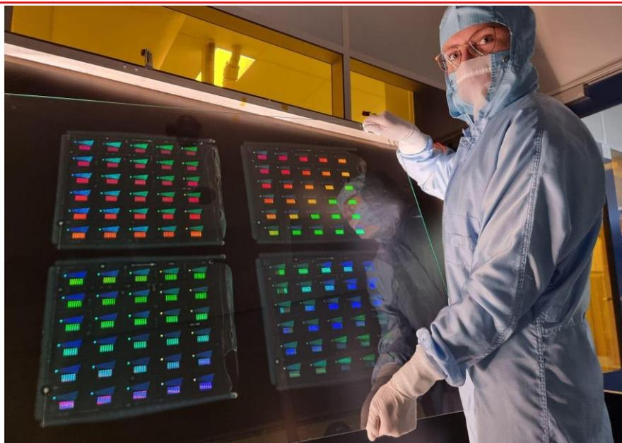
Figure 6. Replication of the 30-up scaled-up sub-master on 4 single wafers in one imprint pass.
