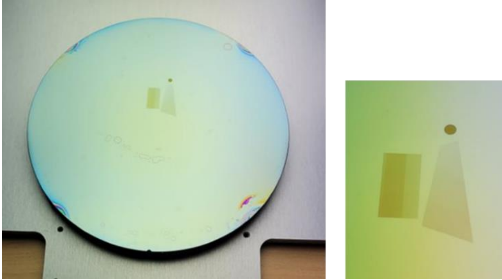
Figure 9 Picture of the waveguide imprint made with a solvent-based resin on a silicon wafer using R2P technology
