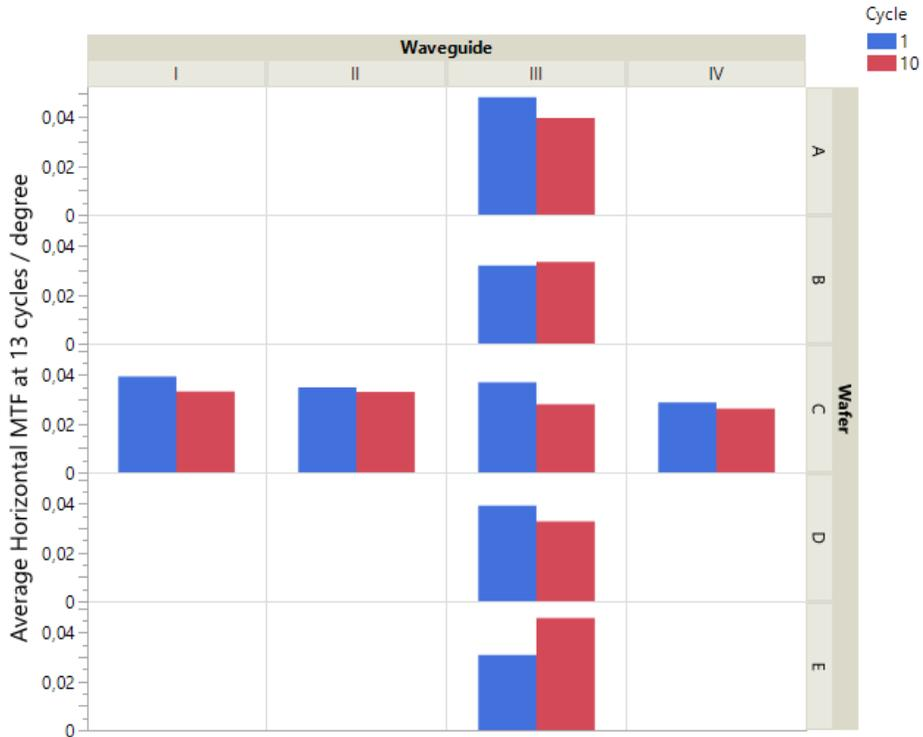
Figure 15 Image quality results from all measured samples with STF1 resin. All measurements were performed with green light in the same eye-box location.
