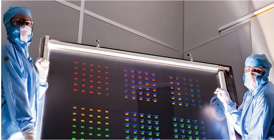
Replication of the 30-up sub-master on 9 single wafers producing 270 waveguides in one imprint pass. Photo credit: Morphotonics
