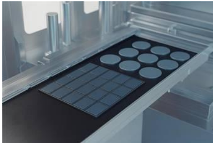
Figure 2 Comparison of wafer layouts on equal-sized Gen3 carriers ( 620 \text{ mm} \times 650 \text{ mm} ): left shows 20 rectangular panels ( 5 \times 4 grid, 151 \text{ mm} \times 120 \text{ mm} ), right shows 9 round wafers ( 3 \times 3 grid, 200 mm diameter). The rectangular format more than doubles eyepiece count per imprint cycle and achieves significantly higher area utilization ( \sim 89.9\% vs. \sim 70.2\% ), enabling improved throughput and reduced material waste.
