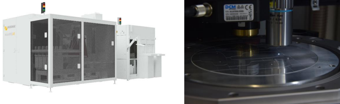
Figure 6 Left: MicroPOLAR machine including SEMI Compliant wafer loadports and customized eyepiece to tray handling unit, Right: High Index-Glas Wafer (diameter 200 mm) on carrier with pre-singulated Eyepieces
